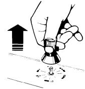
First make sure knobs are set on OFF then pull knob straight off.
