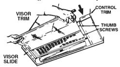
Slide the glass into the visor slides, above each visor clamp (see the illustration in step 14). Align the visor trim and tighten the thumb screws to secure the glass.
