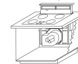
**Note:** Telescopic downdraft vents are not recommended to be installed with cooktops that are flush mounted.
