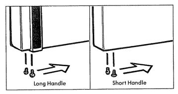
(a) Transfer two screws in bottom left of door to opposite side. (Wait until handle is moved before reinstalling front screw.)
