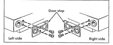
(a) Remove metal doorstop on bottom right of each door.
