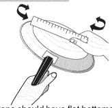
Pan's should have flat bottoms. Check for flatness by rotating a ruler across the bottom. There should be no gaps between the pan and ruler.
