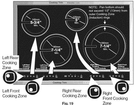
**NOTE:** If a pan made of the correct material is centered properly on any of the active Cooking Zones but is TOO SMALL, the affected Cooking Zone LED will display an F code and the pan will not heat.
