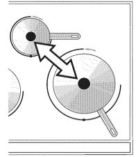
Right-hand Cooking Zones section Your cooktop is equipped with four induction elements within two heating sections. The right-hand and left-hand Cooking Zones are powered by two independent induction inverters - one inverter for each of the two heating sections. Two Cooking Zones in a heating section share the power of one inverter. This is called Power Sharing.
