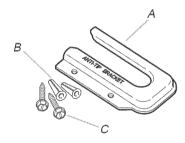
A. Anti-tip Bracket B. Plastic anchors (2)
