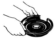
3. **Hold** the surface unit as level as possible with the terminal just started into the receptacle.
