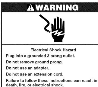
Observe all governing codes and ordinances. A 120 Volt, 60 Hz, AC only, 15- or 20-amp fused electrical supply (or circuit breaker) is required. (A time-delay fuse or circuit breaker is recommended.) It is recommended that a separate circuit serving only this appliance be provided.
