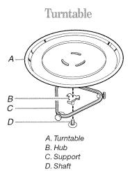
The turntable can rotate in either direction to help cook food more evenly. Do not operate the oven without having the turntable in place. See "Assistance or Service" to reorder any of the parts.
