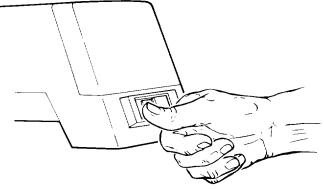
d. WARNING: THIS LOCKING FEATURE IS PROVIDED TO HELP PREVENT UNAUTHORIZED USE OF YOUR SAW. ALWAYS REMOVE THE KEY AND KEEP IT IN A SAFE PLACE. TO REMOVE KEY, HOLD THUMB ON END OF LEVER TO KEEP SWITCH IN "OFF" POSITION AND PULL KEY STRAIGHT OUT.
