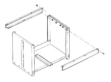
11. Secure rear of lower shelf to right side and left side panels using two (2) 1/4-20 x 1/2 truss head bolts, lockwashers and hex nuts. Hand tighten nuts only at this time.
