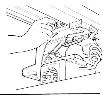
To adjust the carriage bearings perform the following steps.
