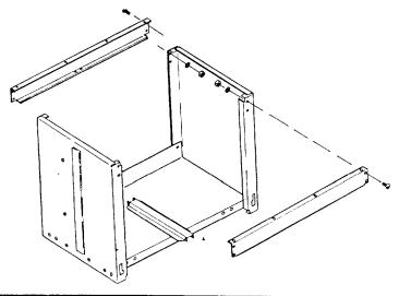
10. Secure rear of lower shelf to right side and left side panels using two (2) 1/4-20 x 1/2 truss head bolts, lockwashers and hex nuts. Hand tighten nuts only at this time.
