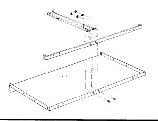
Locate lower support and assemble lower support, shelf and under shelf support with four (4) 1/4-20 x1/2 truss head bolts, lockwashers, and hex nuts.
