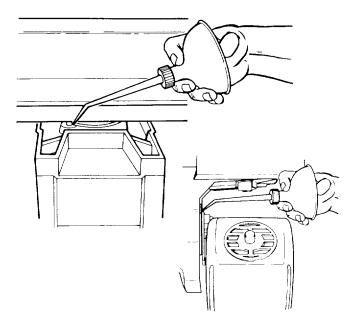
Lubricate the bearing points where the arm attaches to the column tube. With a #2 phillips screwdriver remove two screws and the rear arm cover for access to these points. Be careful not to get lubricant on the locking rings as this will adversely affect the miter locking function.
