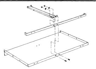
5. Locate lower support and assemble lower support, shelf and under shelf support with four (4) 1/4-20 x 1/2 truss head bolts, lockwashers, and hex nuts.
