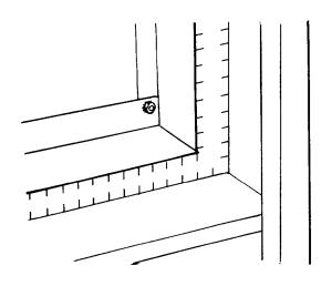
Place square at top side of cabinet and adjust stand so square touches both skirt and side panel (as illustrated). Then tighten right side of front and rear skirts to side panel. Repeat procedure for left side.
