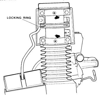
The thread on the elevation shaft assembly can be lubricated through the oil hole in the center of the radial arm cap. Lubricate ramp on the swivel index spring.
