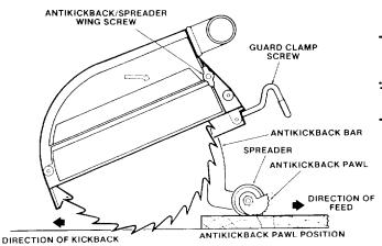
it violently toward the nose of the guard (infeed side of the tool) possibly pulling your hand with it before you can react. See Danger label on outfeed side of the guard just below the dust elbow.
