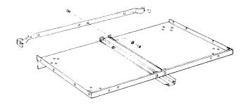
7. Locate the four (4) corner brackets and use eight (8) 1/4-20 x 1/2 truss head bolts, lockwashers and hex nuts to mount the corner brackets to the shelf AS ILLUSTRATED. Tighten the nuts with a 7/16" wrench or socket.
