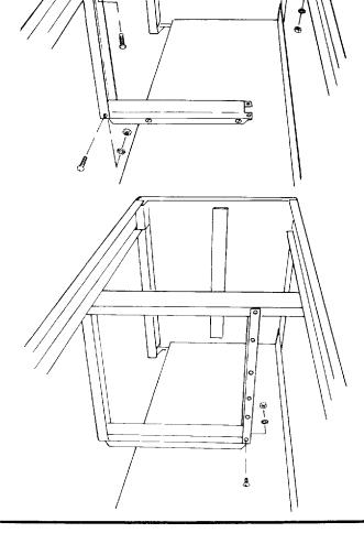
5. Assemble a rear support to each side panel with four (4) 1/4-20 x 1/2 truss head bolts, lockwashers, and hex nuts. Tighten nuts securely. Rear support must touch lower shelf for holes to line up with front holes.
