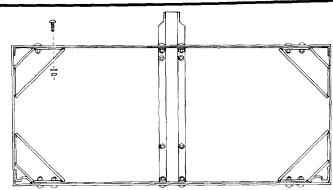
8. Locate the right and left foot assemblies, two (2) leveling feet, two (2) 1/2-13 hex nuts, the right and left side panels, and four (4) 1/4-20 x 7/16 slotted truss head bolts. Attach the R.H. foot assembly to the right side panel in holes as illustrated. Repeat procedure with L.H. foot assembly to left side panel.
