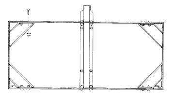
8. Locate the right and left side panels and eight (8) 1/4-20 x 1/2 truss head bolts, lockwashers and hex nuts to attach side panels to shelf. Mount the bolts through the four holes as illustrated and tighten with 7/16 wrench or socket. To assemble, lay the side panel on its backside and stand the shelf up as illustrated.
