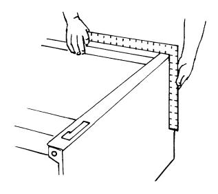
WARNING: TO AVOID INJURY FROM UNEXPECTED SAW OR WORK MOVEMENT, LEVELING FEET MUST BE ADJUSTED SO THAT SAW DOES NOT ROCK. TO AVOID UNEXPECTED CARRIAGE MOVEMENT, ADJUST LEVELING FEET SO THAT THE ARM SLOPES SLIGHTLY DOWNWARD TO THE REAR.
