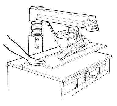
Use of the molding head in the horizontal position also requires the proper accessory guard be used (see recommended accessories page 57).
