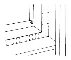
2. Place square at top side of cabinet and adjust stand so square touches both skirt and side panel (as illustrated). Then tighten right side of front and rear skirts to side panel. Repeat procedure for left side.
