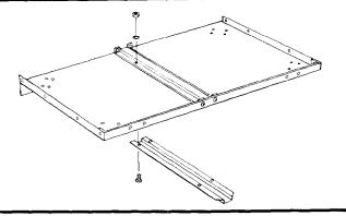
6. Attach the second shelf stiffener to the under support. Use two (2) 1/4-20 x 1/2 truss head bolts, lockwashers, and hex nuts to fasten to the under support with 7/16" wrench or socket.
