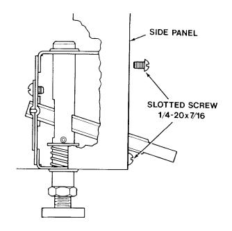
9. Locate the right and left side panels and eight (8) 1/4-20 x 1/2 truss head bolts, lockwashers and hex nuts to attach side panels to shelf. Mount the bolts through the four holes as illustrated and tighten with 7/16 wrench or socket. To assemble, lay the side panel on its back side and stand the shelf up as illustrated.
