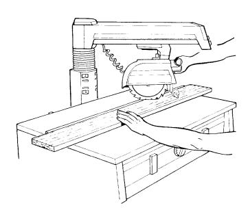
rectangular frame. The radial arm is set to a desired angle of cut, swivel and bevel settings at 0° and locked. The workpiece being cut is positioned and held firmly against the fence and the carriage pulled forward along the radial arm just far enough to complete the cut. Carriage should then be returned to the full rear position and locked. Allow the saw blade to come to a stop before removing the workpiece from the saw table.
