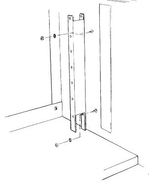
6. Locate the twelve (12) stand slide brackets, twenty-four (24) truss head bolts, lockwashers and hex nuts. Assemble the stand slide brackets on the rear supports and inside of the side panels in holes as illustrated. Assemble the stand slide brackets on the center and rear supports in holes as illustrated starting at the top.
