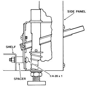
13. Locate the four (4) swivel casters and sixteen (16) 1/4-20 x 7/16 slotted truss head bolts, lockwashers, and hex nuts. Line up the caster with the matching holes in lower shelf and corner bracket (shaded area). Attach the caster with four (4) slotted truss head bolts, lockwashers and hex nuts and tighten by hand as illustrated. When all four bolts are installed use a regular screwdriver and a 7/16" wrench or socket to tighten securely. Repeat procedure for the three remaining casters.
