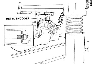
**NOTE:** Make sure bevel encoder lines up with actuator on top of motor. Bevel encoder cord should be positioned between actuator on motor plate. Slide encoder to top of scale if adjustment is needed.
