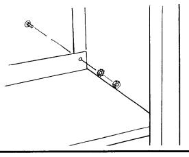
12. Lay the stand on the backside, locate two (2) spacers, two (2) 1/4-20 x 1" truss head bolts, lockwashers and hex nuts. Assemble the spacers between each of the foot assemblies and the lower shelf on each side with one (1) truss head bolt, lockwasher and hex nut each as illustrated. Hand tighten nut.
