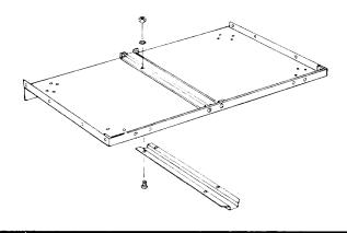
6. Attach the second shelf stiffener to the under support. Use two (2) 1/4-20 x 1/2 truss head bolts, lockwashers, and hex nuts to fasten to the under support with 7/16" wrench or socket.
