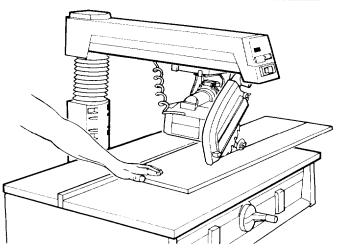
board against the fence must be straight and will not catch on kerfs in the fence - for workpieces thicker than the fence is high, install a higher fence (at least the thickness of the workpiece). NEVER RIP "FREEHAND" (without aid of fence).
