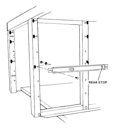
Locate the twelve (12) center slide brackets and the two (2) lubrication packets. Lubricate upper & lower channel on all twelve (12) center slide brackets.
