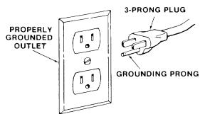
This power tool is equipped with a 3-conductor cord and grounding type plug which has a grounding prong, listed by Underwriters' Laboratories. The ground conductor has a green jacket and is attached to the tool housing at one end and to the ground prong in the attachment plug at the other end.
