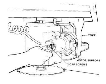
**NOTE:** It may be necessary to use pliers to grip the short end of the Hex "L" wrench to loosen or tighten the socket cap screws. Remember to wear eye protection when performing this procedure.
