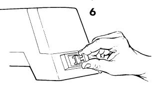
b. To turn switch on, insert finger under end of switch lever and pull end out.
