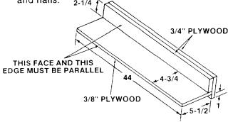
b. **Make the push block** using a piece of 3/8" and 3/4" plywood.
