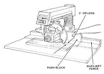
DO NOT USE NAILS. This is to prevent dulling the sawblade in the event you cut into the push block.
