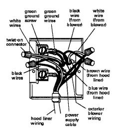
Connect both green ground wires (from exterior blower motor and from 120-volt supply wiring) under the unused green ground screw.
