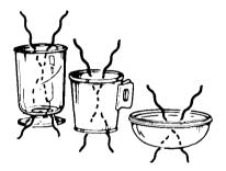
Microwaves pass through glass, paper and plastic without heating them so food absorbs the energy. Microwaves bounce off metal pans so food does not absorb the energy.
