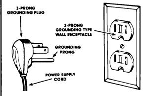
polarized 3-prong grounding plug. It must be plugged into a correct polarized mating 3prong grounding type wall receptacle, properly installed and grounded in accordance with the National Electrical Code and local codes and ordinances. If a mating wall receptacle is not available or if you are not sure if the wall receptacle is properly grounded and polarized, have it checked by a qualified electrician.
