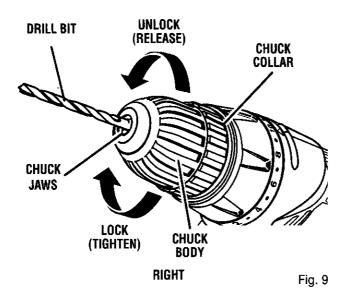
■ To tighten: grasp and hold the collar of the chuck with one hand, while rotating the chuck body with your other hand.
