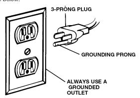
This power tool is equipped with a 3-conductor cord and grounding type plug, approved by Underwriters Laboratories and the Canadian Standards Association. The ground conductor has a green jacket with or without yellow stripes and is attached to the tool housing at one end and to the ground
