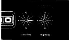
3. Push in and turn the Start Time Knob clockwise to the time you want baking to start.
