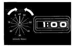
Let the Minute Timer Knob pop out. Turn in either direction until Minute Timer hand points to OFF. The clock setting will change if you push in the knob when turning.
