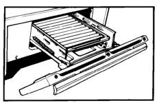
**1.** Pull the broiler drawer open and tilt the door panel down.
