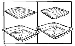
Place broiler pan grid so grease can drain down sides into lower part of broiler pan. See picture.
