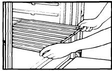
Position the racks properly before turning on the oven. To change rack position, pull rack out to stop, raise front edge and lift out. The rack(s) should be placed so the top of the food will be centered in the oven. Always leave at least 1½ to 2 inches (4-5 cm) between the sides of the pan and the oven walls and other pans.
