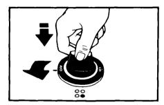
Control knobs must be pushed in, then turned to LITE position. The clicking sound is the ignition sparking.
