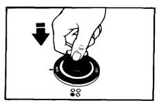
**4.** Push control knobs straight back on. Make sure they point to OFF.
