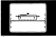
During baking, the oven burner will turn on and off to maintain the temperature setting.
