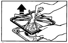
2. Lift off grates and remove the reflector pans.
