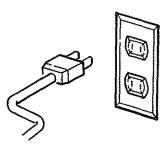
This power tool is equipped with a 2-conductor cord listed by Underwriters Laboratories (UL). The plug permits you to use any conventional 120-volt electrical
