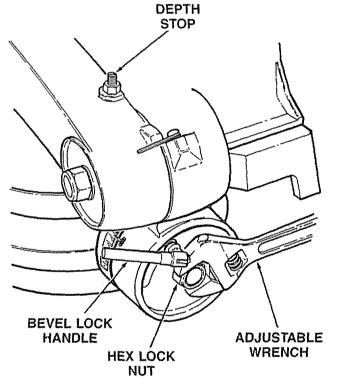
Lower the blade into the slot of the turn table. Check blade clearance and maximum cutting distance (distance from fence where blade enters) to front of turn table slot. Readjust if necessary.
