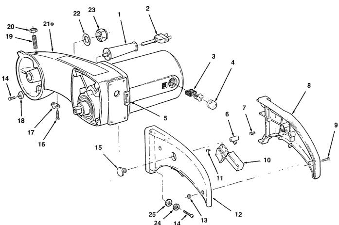
Always order by Part Number—Not by Key Number FIGURE 2—ARM AND MOTOR ASSEMBLY
