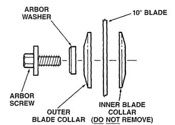
WARNING: AFTER INSTALLING A NEW BLADE, MAKE SURE THE BLADE CLEARS THE TABLE SLOT AT THE 0° AND 45° BEVEL POSITIONS. LOWER THE BLADE INTO THE LOWER TABLE AND CHECK FOR ANY CONTACT WITH THE BASE OR TURN TABLE STRUCTURE.
