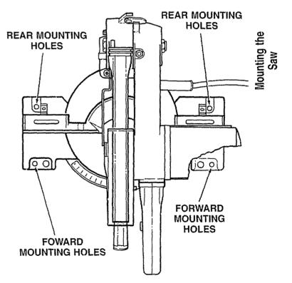
**NOTE:** Fence has been moved forward for access to rear mounting holes.
