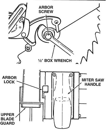
**NOTE:** Pay attention to pieces removed, noting their position and direction they face (see illustration). Wipe the blade collars clean of any sawdust before installing the new blades.
