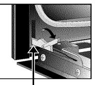
Lock engaged for door removal
