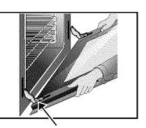
HINGE SLOT Door removed from the wall oven
