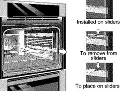
Pull oven rack forward and lift it up off the oven rack slider.
