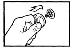
Push control knobs straight back on. Make sure they point to OFF.
