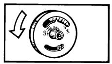
To lower the temperature, move the pointer to the left. Each notch equals about 10°F (5°C).
