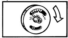
**4.** To raise the temperature, move the pointer to the right. Each notch equals about 10°F (5°C).
