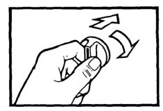
Surface element control knobs must be pushed in before turning. Turn either way until setting you want shows in window. Set them anywhere between HI and OFF.
