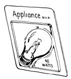
3. Remove the light bulb from its socket. Replace the bulb with a 40-watt appliance bulb.
