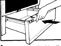
Lift drawer front and push in until metal stops on drawer slide rails clear white stops on drawer guides. Lift drawer front again to clear second stop and slide drawer closed.
