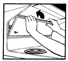
4. With both hands, carefully fit the glass light cover into the bottom metal support trim. Replace the top support trim and screw.
