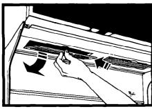
To remove each filter, place thumb in the indentation at the center front of the filter. Push back and pull down.
