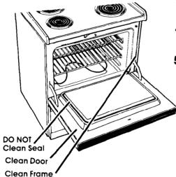
DO NOT clean the fiberglass seal. DO NOT move it or bend it. Poor cleaning and poor baking will result.
