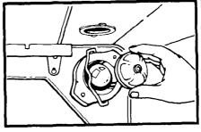
2. Remove the bulb cover in the back of the oven by pulling out and pushing the wire holder to the side.
