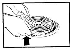
Lift the edge of the element, opposite the receptacle, just enough to clear the reflector bowl.
