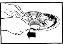
**3.** Pull the surface element straight away from the receptacle.
