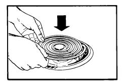
4. Push the surface element terminal into the receptacle. When the terminal is pushed into the receptacle as far as it will go, the surface element will fit into the reflector bowl.
