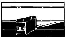
When the Lock Light is off and the oven is cool, move the Lock Lever to the left. Do not force it. Wait until it moves easily.
