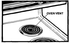
**Do not block the vent.** Poor baking can result.
