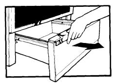
Pull drawer straight out to the first stop. Lift front and pull out to the second stop.
