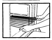
Position the rack(s) properly before turning on the oven. To change rack position, pull rack out to stop, raise front edge and lift out. The rack(s) should be placed so the top of the food will be centered in the oven. Always leave at least 1½ to 2 inches (4-5 cm) between the sides of the pan and the oven walls and other pans. For more information, see the "Cooking Guide"
