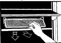
To remove filter, lift vent door. Use plastic tab at center of the filter to push up and lift out the filter.
