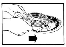
Hold the surface element as level as possible with the terminal just started into the receptacle.
