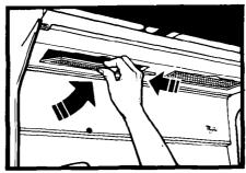
To replace, place the long edge of the filter against the clips at the back of the opening. Push filter back and up until it snaps into place.
