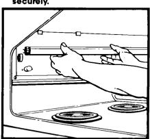
3. Grasp the fluorescent lamp at both ends. Roll bottom of the lamp towards the front until both ends come out of the receptacles. Replace with a 24-inch, 18- or 20-watt cool-white fluorescent lamp. If starter needs replacement, push in and turn to remove and replace.
