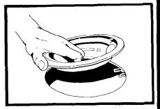
2. Line up opening in the reflector bowl with the surface element receptacle.
