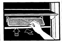
2. To replace, place top edge of the filter against the clips at the top of the opening. Push up and in until filter snaps in place. Make sure the plastic tab at the bottom of the filter is facing out.
