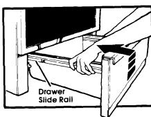
Fit ends of drawer slide rails into the drawer guides on both sides of opening.
