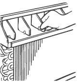
Remove the front grille to adjust the vertical louvers side-to-side to direct the air left or right.
