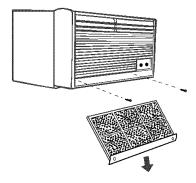
3. Pull the grille out from the bottom and lift up from the tabs on the top of the case.
