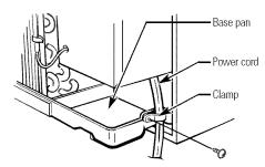
When the wall outlet is to the left, extend the cord under the unit and hold it in place with the clamp.
