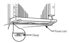
Attach the front grille. An opening for the power cord is on the bottom of the front grille.
