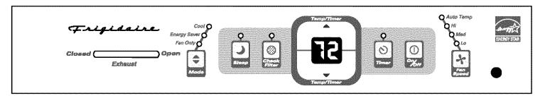
This Exhaust Control allows the air conditioner to either recirculate inside air (CLOSED) or exhaust air to the outside (OPEN). The CLOSED position is used when maximum cooling is desired. It may also be used for air recirculation without cooling when the air conditioner is set in any FAN position.
