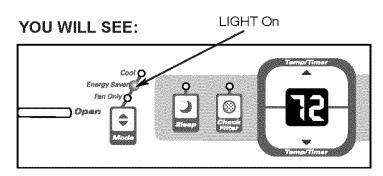
Note: In this mode, the fan will continue to run for 3 minutes after the compressor shuts off. The fan then cycles on for 2 minutes at 10 minute intervals until the room temperature is above the set temperature, at which time the unit turns back on.
