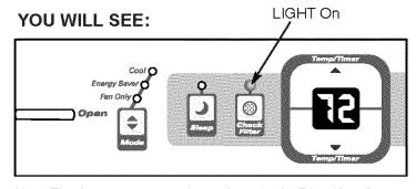
Note: This feature is a reminder to clean the Air Filter (See Care and Cleaning) for more efficient operation and cooling. The LED (light) will illuminate after 250 hours of operation. To reset after cleaning the filter, press the "Check Filter" button and the light will go off.
