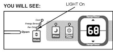
Note: Use this function only when cooling is not desired, such as for room air circulation or to exhaust stale air (Remember to open the vent during this function, but keep it closed during cooling for maximum cooling efficiency). You can choose any fan speed you prefer.
