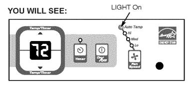
Note: Fan speed starts at high and adjusts to a slower speed as the room temperature dictates. For example, if the room doesn't get too warm it will stay at the slowest speed. If the room temperature rises quickly, such as a door being opened, it will automatically go to the highest speed. The fan speeds will readjust back to the slowest speed as the room returns to the original set temperature. Press the Fan Speed button to adjust the fan speed manually.
