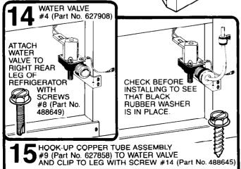
**Connect Water Line** Between Water Valve (At The Bottom) To Inlet Tube
