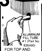
BOTTOM MOUNT FREEZER SLIP TUBE #1 (Part No. 836490) OVER WATER INLET TUBE—PUSH ON
