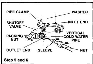
6. Slip compression nut and compression sleeve on copper tubing as shown in diagram. Insert end of tubing into outlet end squarely as far as it will go. Screw compression nut to outlet end with adjustable wrench. Do not overtighten. Turn ON main water supply and flush out tubing until water is clear. Turn
