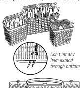
evenly. Small plastic items, such as measuring spoons and lids from small containers should go in the bottom of the silverware basket with the silverware on top. The one-piece silverware basket (on some models) can be placed in the front, right
