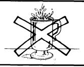
Liquids heated in certain containers (especially cylindricalshaped containers)may become overheated. The liquid may splash out with a loud noise during or after heating or when adding ingredients (coffee, etc.) resulting in harm to the oven and possible personal injury. For best results stir any liquid several times before heating or reheating.
