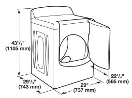
**NOTE:** Most installations require minimum 5" (127 mm) clearance for exhaust vent with elbow. See "Venting Requirements."
