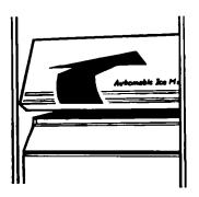
Lift the signal arm so it clicks into the OFF (up) position. Ice can still be dispensed, but no more can be made.
