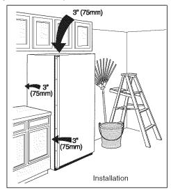
**NOTE:** The exterior walls of the refrigerator may become quite warm as the compressor works to transfer heat from the inside. Temperatures as much as 30° F warmer than room temperature can be expected. For this reason it is particularly important in hotter climates to allow enough space for air circulation around your refrigerator.
