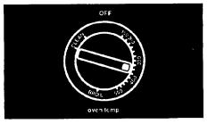
3. Set the Oven Temperature Control to the temperature you want. The Oven HEATING Indicator Light will come on. The oven is preheated when the Oven HEATING Indicator Light first goes off.
