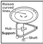
Place the support (Part No. 4393752) on the cavity bottom.
