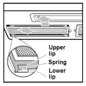
6. To replace grease filters, slide filter in the frame slot on one side of the opening. **Push** filter upward and **push** to the other side to lock into place.
