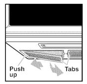
**3. To remove the charcoal filters,** push the back of each filter away from you. This will slide the front of the filter off the lower lip. Swing the front of the filter down and slide the filter out.
