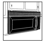
3. Tip the grille forward, then lift out to remove.
