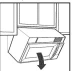
oven downward. (Be careful that door does not swing open.) Lift off the support tabs **G** at the bottom of the mounting plate. Set the microwave oven aside on a protected surface.
