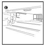
combination in place with one hand. Pull hook (3) to release microwave hood from mounting plate. If grille cannot be removed (per instructions in Step 2.), insert a thin looped wire or similar tool through an opening in grille to pull hook.
