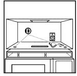
turntable and support, tape the door in the closed position. Then remove the two bolts **D** securing the microwave oven to the upper cabinet.
