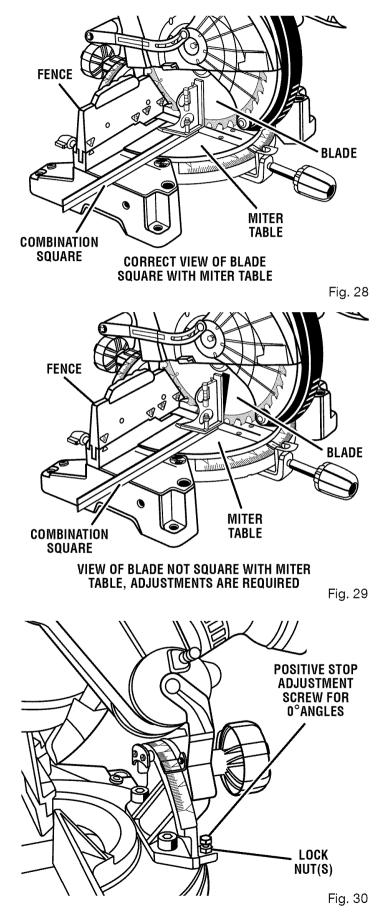
This saw has two scale indicators, one on the bevel scale and one on the miter scale. After squaring adjustments have been made, it may be necessary to loosen the indicator screws and reset them to zero.
