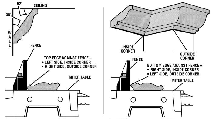
**CROWN MOLDING FLAT ON MITER TABLE**
