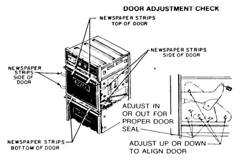
Place 2'x 18" strips of newspaper in locations indicated by illustration. Allow one end of the paper to extend into the oven cavity. Pull gently at each piece of paper. If door is properly adjusted, each piece of paper will offer firm resistance when pulled. When door is out of adjustment, slide unit out far enough to expose hinges on each side (see preceding page). Loosen screws and move bottom of door to a proper fit. After completing adjustment tighten all screws in hinges.
