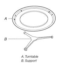
The turntable can rotate in either direction to help cook food more evenly. Do not operate the oven without the turntable in place. See "Assistance or Service" to reorder any of the parts.
