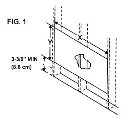
Carefully measure and cut an opening with the following dimensions, See FIGS. 1 and 2.
