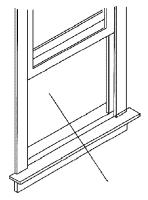
Place cabinet in window with bottom stool angle firmly seated over window stool as shown. Bring window down temporarily behind top angle to hold cabinet in place.
