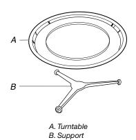
The turntable can rotate in either direction to help cook food more evenly. Do not operate the oven without the turntable in place. See "Assistance or Service" to reorder any of the parts.
