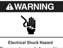
Disconnect power before making electrical connections.
