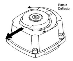
Figure 4 - Exhaust Deflector Adjustment
