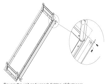
Square the unit and wrench tighten all fasteners.
