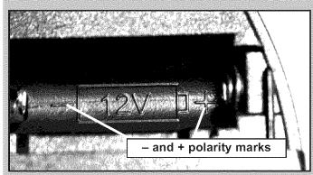
FIG. 8-2 Match battery polarity.
