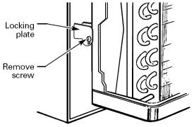
Remove and discard the shipping screw on the back of the air conditioner to allow removal of the air conditioner from the case.
