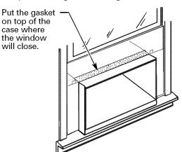
Place the vinyl window gasket over the case top gasket. Insert the panel tabs through the slits in the gasket. Cut the gasket on each side to the width of the window.
