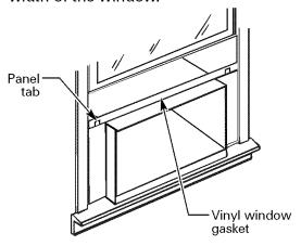
Close the window tightly on the vinyl gasket. Bend the gasket forward to expose the panel tabs. Drill pilot holes into the window sash.
