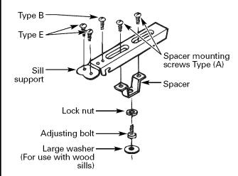
Before attaching the sill supports, place them on the window stool. Select the spacer position that will place the spacer near the outermost point on the sill. Tighten the spacer mounting screws.
