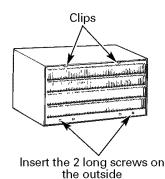
If attaching the grille on the inside of the case use the 2 short screws.
