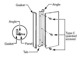
Install the panels in the window. Place the spring clips 3" from the top and the bottom. Squeeze and push the clips to fit in the window track and the tab into the sill support.
