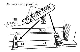
Turn the bolts and tighten the lock nuts to make the sill supports level or tilt down 1/8" to the outside. Line up the "V" notch with 12%" marks. Drill pilot holes and attach the sill supports.
