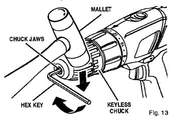
Open chuck jaws and remove hex key. Remove the chuck screw by turning it in a clockwise direction. See Figure 14.
