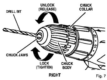
To tighten the chuck jaws on drill bit; grasp and hold the collar of the chuck with one hand, while rotating the chuck body with your other hand.
