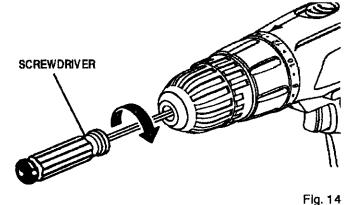
Insert hex key in chuck and tighten chuck jaws securely. Tap sharply with a mallet in a counterclockwise direction. This will loosen chuck on the spindle. It can now be unscrewed by hand. See Figure 15.
