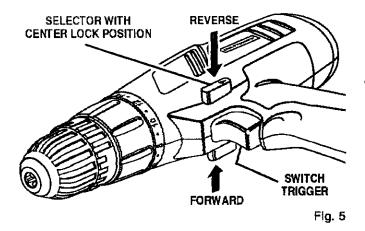
WARNING: Battery tools are always in operating condition. Therefore, switch should always be locked when not in use or carrying at your side.
