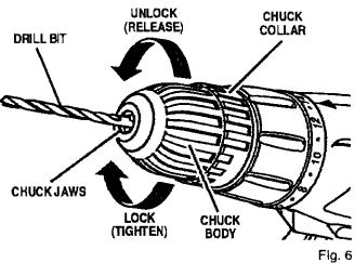
WARNING: Do not hold chuck body with one hand and use power of the drill to tighten chuck jaws on drill bit. Chuck body could slip in your hand or your hand could slip and come in contact with rotating drill bit. This could cause an accident resulting in serious personal injury.
