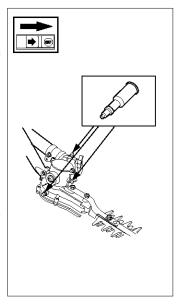
The lubricant in the gearbox does not normally need to be replaced other than with repair.
