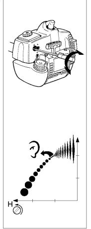
when the machine 'splatters' a little . If the machine smokes heavily at the same time as it 'splatters' heavily the adjustment is too rich.
