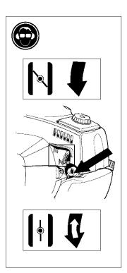
Press the machine body against the ground using your left hand (NOTE! Do not use your foot). Grip the starter handle with your right hand and slowly pull the starter cord out until you feel some resistance, (the starter hooks grip) now quickly and powerfully pull the cord. Immediately press the choke control in when the engine fires and repeat until the engine starts. When the engine starts, quickly apply full throttle and the start throttle will automatically disengage.
