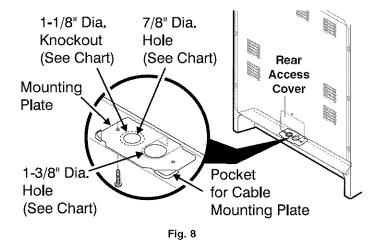
Range Connection Opening Size Chart Supply Cord Kit ampere rating information. See serial plate on range for kilowatt rating data. See Serial Plate on Range for Cord Kit Diameter (inches) of Range KW Rating Ampere connection Opening Rating Permanent Cord Kit 120/240 Volts 120/208 Volts Wiring 8.8-16.5 KW 7.9-12.5 KW 1-3/8 in. 1-1/8 in. 40/50 Amp 16.6-22.5 KW 12.6-18.5 KW 50 Amp 1-3/8 in. 1-3/8 in.
