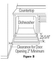
**Note:** ADA installation,  $(32 \cdot 1/2'')$  beneath 34" high counter-tops may be accomplished by adjusting the toekick and leveling legs.
