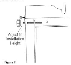
Measure installation height and dishwasher height. Extend leveling legs out from the dishwasher base, 1/4" less than installation height.
