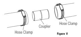
Secure the drain hose to the air gap, waste tee or disposer with clamps.
