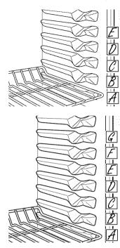
30" Trivection™ oven has 5 rack positions A–E (as shown). 30" lower oven of double oven has 7 rack positions A–G (as shown).
