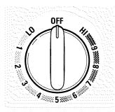
At both OFF and HI the control clicks into position. You may hear slight clicking sounds during cooking, indicating the control is maintaining your desired setting.
