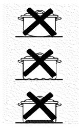
Pans with rounded, curved, ridged or warped bottoms are not recommended.
