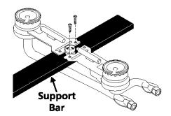
To clean, soak the burners in a 1:1 solution of ammonia and water for 30 to 40 minutes. For stubborn stains, scrub with soap and water or a mild abrasive cleanser and a damp cloth. Dry the burners thoroughly in a warm oven for 30 minutes. Then replace them, making sure they are properly seated and level. **DO NOT** wash burner units in the dishwasher.
