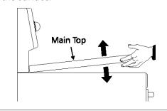
on when the cooktop is raised for cleaning. Be sure that the top is completely lowered and securely in place before turning on the burners.
