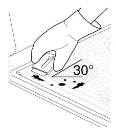
If soils remain, carefully scrape soils with a metal razor blade scraper, holding scraper at a 30 degree angle to the surface. Remove loosened soils with cooktop cleaning cream and buff surface clean.
