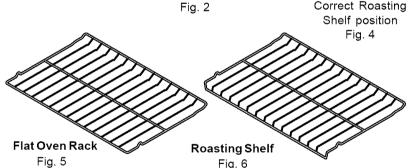
Place **Roasting Shelf** with care in rack position 7 (See Fig. 2). Be sure the Roasting Shelf is level and the front end of the shelf rests over the front ends of the oven rack glides on both sides of the oven interior (See Figs. 3 & 4).
