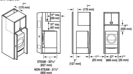
\*Required spacing \*\*For side or bottom venting, 0" (0 mm) spacing is allowed.
