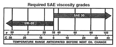
NOTE: Although multi-viscosity oils (5W30, 10W30, etc.) improve starting in cold weather, these multi-viscosity oils will result in increased oil consumption when used above 32° F. Check the engine oil level more frequently to avoid possible engine damage from running low on oil.
