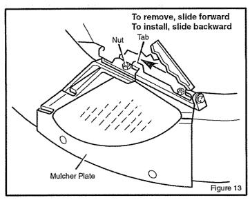
B. Lift the mulcher plate away from the mower housing (Figure 14).
