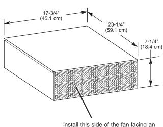
install this side of the fan facing an unoccupied space.
