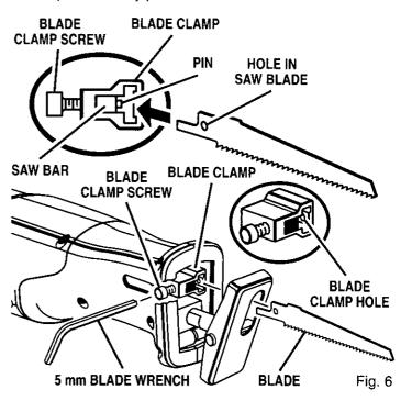
**Note:** There may be times when the blade clamp sticks to the saw bar and will not loosen enough to allow blades to be installed or removed. If this happens, loosen the blade clamp screw with the blade wrench, then tap lightly on the end of the blade wrench with a mallet. See Figure 7.
