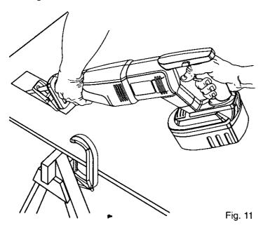
Mark the line of cut clearly. Choose a convenient starting point inside the area to be cut out and place the tip of the blade over that point. Rest front edge of base assembly on work and hold firmly in position. Depress the lock-off button, then pull switch trigger to start the cutting action.
